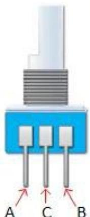
On one side of the switch there are three pins. They are normally referred to as A, B and C. In the case of the KY-040, they are oriented as shown.
