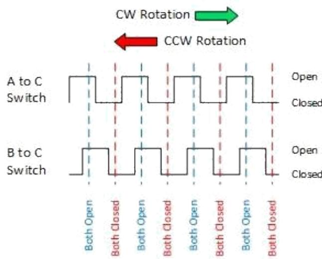
Essentially, determining which switch changed states first is how the direction of rotation is determined.
